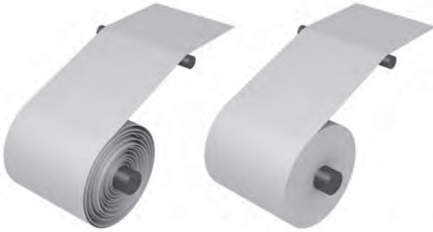
A strip rolled up without EPC Post-processing required
