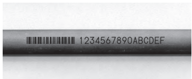
Fig.8 Example of bar code and number printed on steel pipe with LASER MARKER
