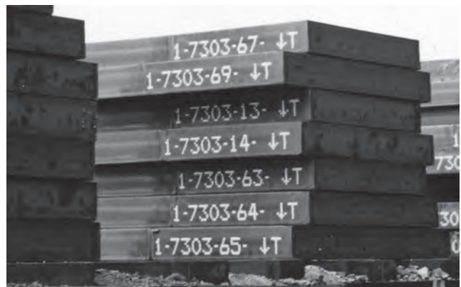
Fig.6 Marking on the side of 300°C - 1000°C slabs using DOT MARKER
