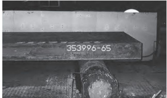
Fig.4 Marking on the side of 600°C - 1000°C slabs using JET MARKER
