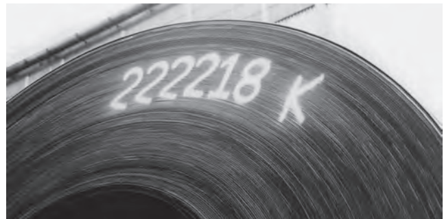
Fig.5 Marking on the side of 600°C - 800°C hot coils using JET MARKER
