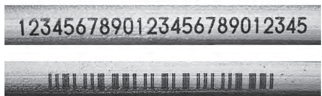
Fig.15 Example of text and ber code on a 6mm think plate
