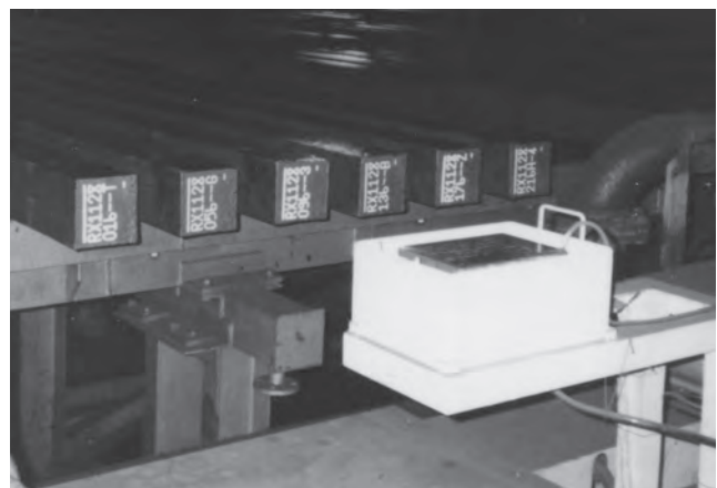
Fig.12 The same marking head marks on billets arranged both vertically and horizontally
