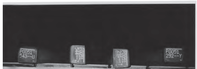
Fig.11 The same marking head marks on billets arranged both vertically and horizontally
