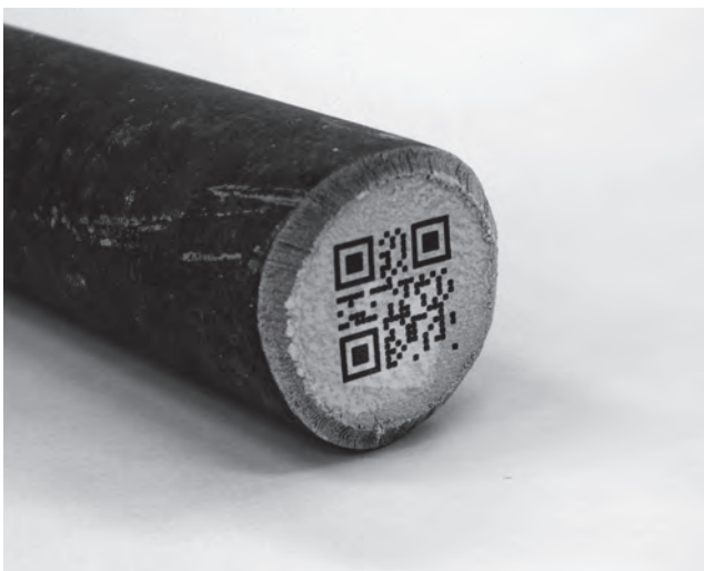
Fig.7 Example of 2D code printed on edge of a steel bar with LASER MARKER
