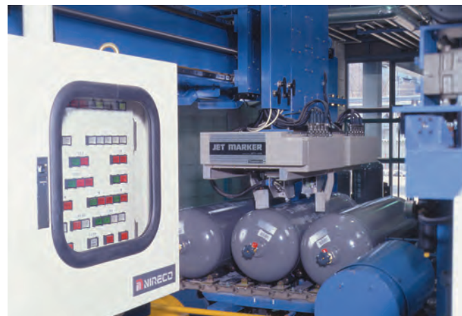
Marking on propane gas cylinders using JET MARKER
