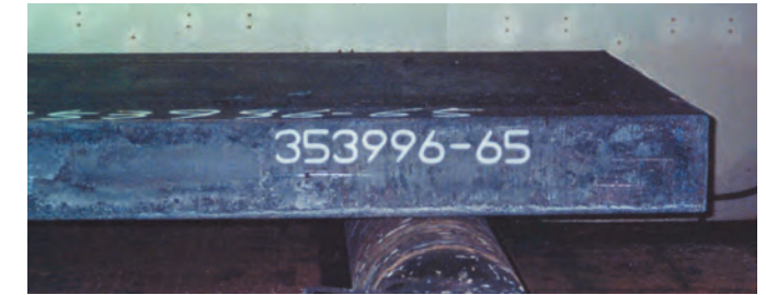
▲ Marking on the side of 600°C to 1000°C slabs using JET MARKER
