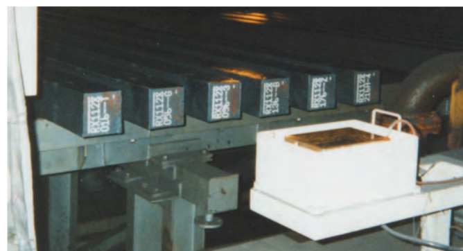
Marking on the end face of 300 to 700 billets using JET MARKER
