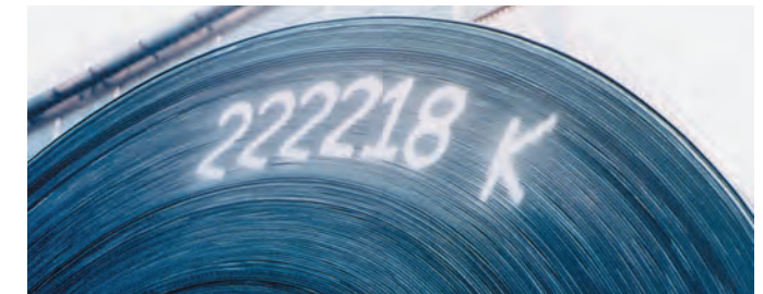
▲ Marking on the sides of 600°C to 800°C hot coils using JET MARKER
