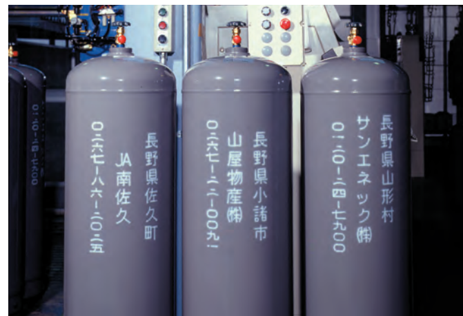
Actual markings performed by the left machine. The marking are customer coded. (Chinese, Hangul, and special characters available)
