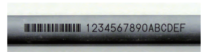
▲ Example of bar code and number printed on steel pipe with laser marker
