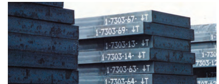
▲ Marking on the side 300°C to 1000°C slabs using DOT MARKER
