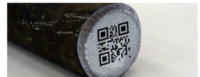
▲ Example of 2D code printed on edge of a steel bar with laser marker
