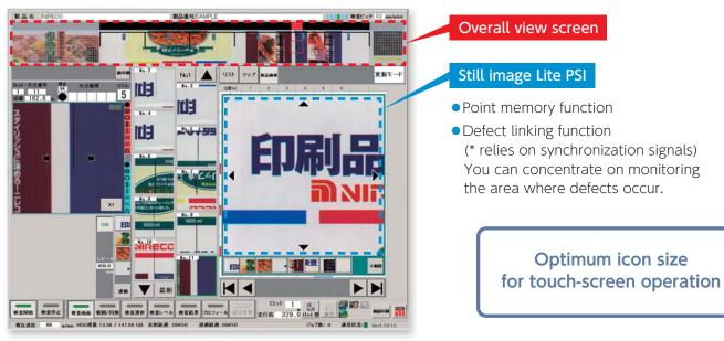
\* Synchronization signals are timed so that the inspection system can make stable inspections (1 pulse per rotation of the plate cylinder).
