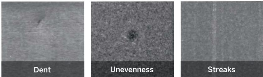
In addition to the ones shown above, the system can also detect defects such as fish eyes, agglomerates, and wrinkle.
