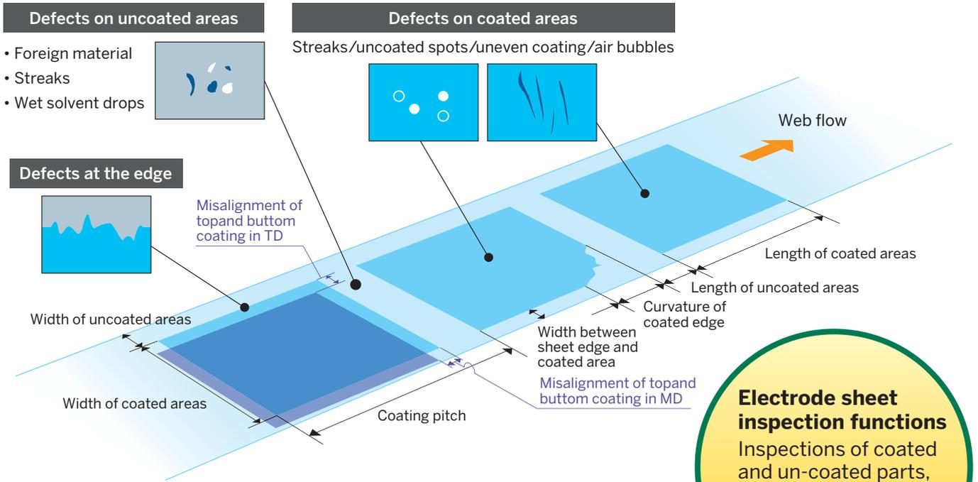
**Electrode sheet inspection functions**
